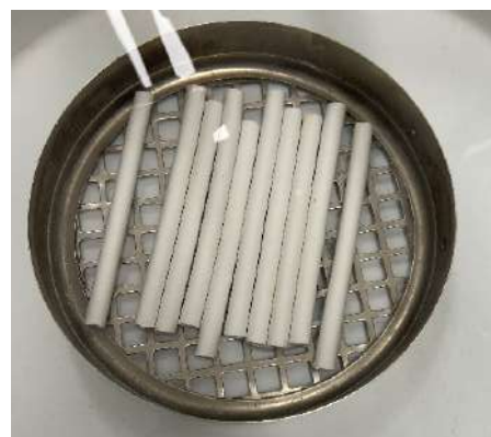
Fig 4. Test bars immersed on 20^{\circ}\text{C} water.
