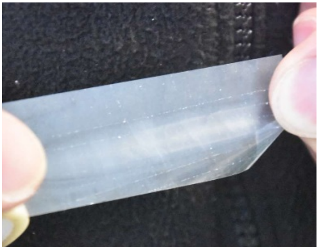
Figure 13: The scotch tape is examined for detached coating particles.
