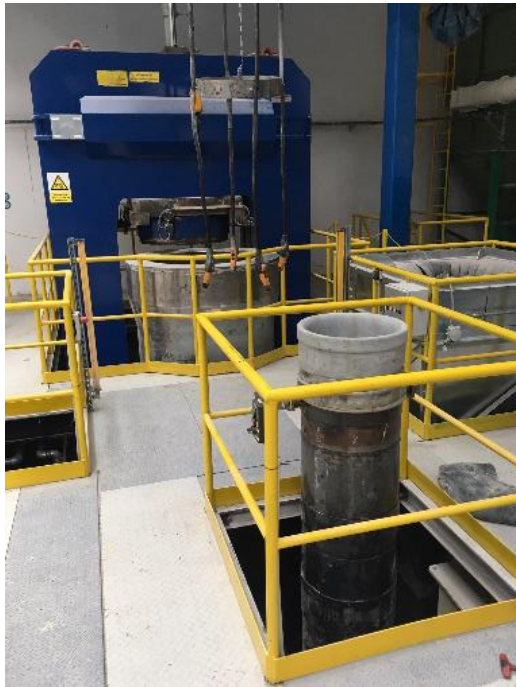
Figure 3: In the front we can see the steel-cylinder with a rubber-cannister inside. Behind we can see the blue structure of the press itself.
