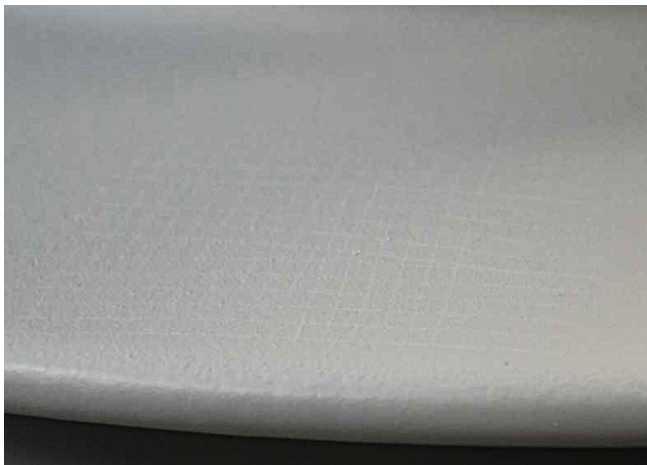
Figure 11: the cross-cut area on the RTV-coating.
