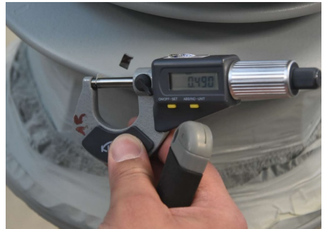
Figure 9: RTV-Silicone coating thickness measurement.
