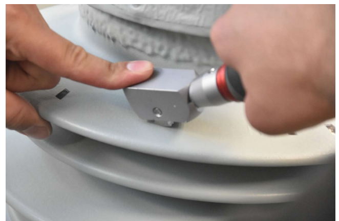
Figure 10: Scratching the coating with a multiblade tool.
