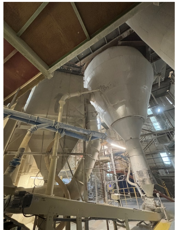
Figure 2: the CAB spray dryer, the manufactured powder is transported with conveyor belts to silos.
