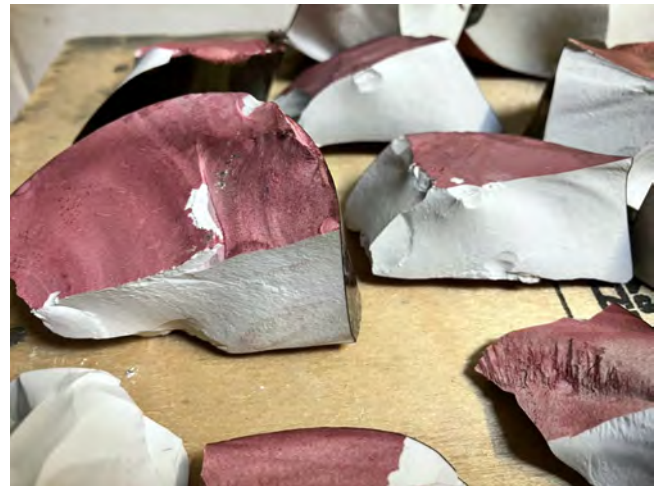
Photo 2: C-130 body pieces on the porosity test samples according to IEC 60383-1 § 26 (10), no porosity.
