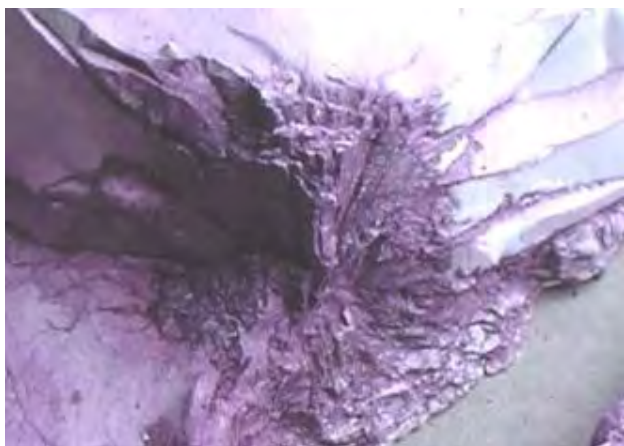
Photo 1: Quartz initiated crack growth in a long rod. Quartz content > 2%
