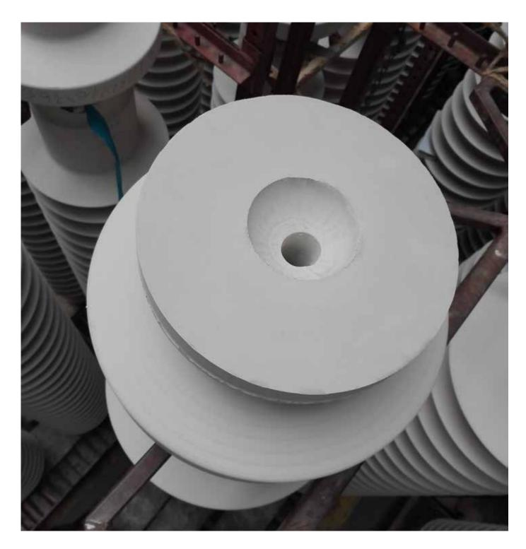
PPC Fiber Optic Hole Post Insulator is available with all standard and non-standard PPC porcelain and hybrid station post insulator types. Ranging up to 2,550 kV BIL and designed for the most challenging performance environments, PPC Fiber Optic Hole Post Insulators are a well-proven solution for digital substations and smart grid's integrated prognostics systems.
