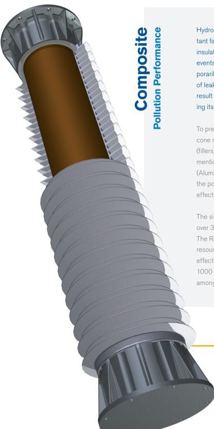
Hydrophobicity is widely considered to be the most important factor regarding the insulation behavior of composite insulators. It is well known that under specific pollution events, the hydrophobicity of silicone rubber can be temporarily inhibited. Such conditions can lead to development of leakage current on the surface of silicone housing, to result in initiation of possible erosion of the silicone housing itself.
