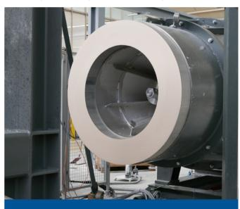
With the new XXL Extruder, PPC Insulators is capable of producing multipart insulators up to 1,100 mm in diameter and exceeding 11,000 mm in length and single piece hollow insulators with 2,750 mm length, ranging from 72 kV up to 1,200 kV AC and 1,100 kV DC,
